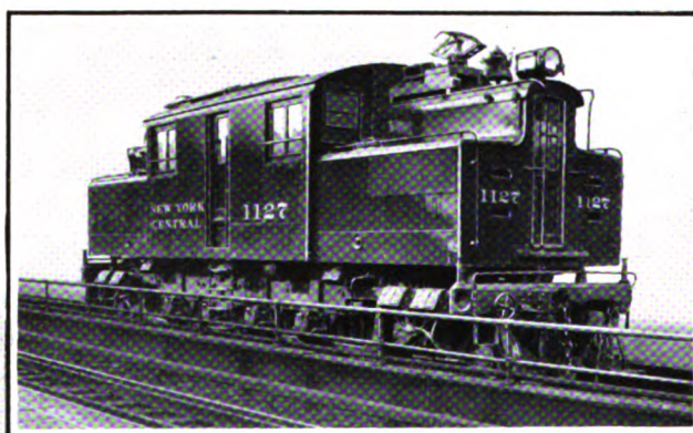
Class S-2 113-ton Locomotive
