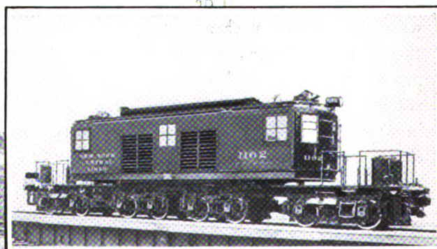
Class T-2 130-ton Locomotive
